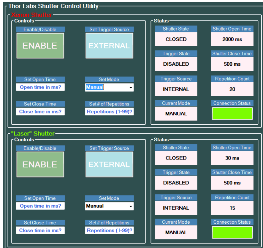
Figure C.1 GOEGUI – ThorLabs Shutter Control Utility. The figure depicts the program after the connection has been made.
